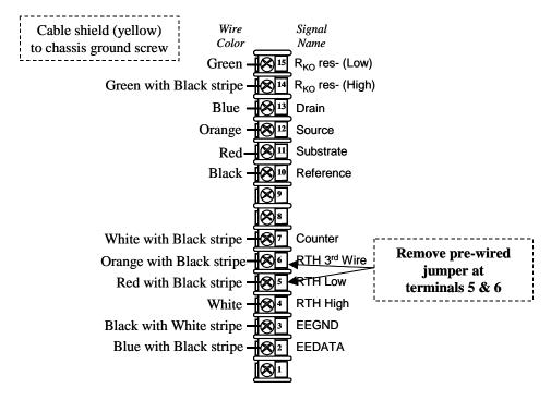
Figure 7-2 Terminal Designations for Durafet III Electrode
